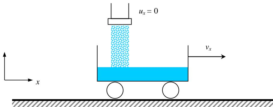
Figure 1. Sketch of the horizontal motion of an open-topped freight car that is filled with water, from a fixed pipe.
