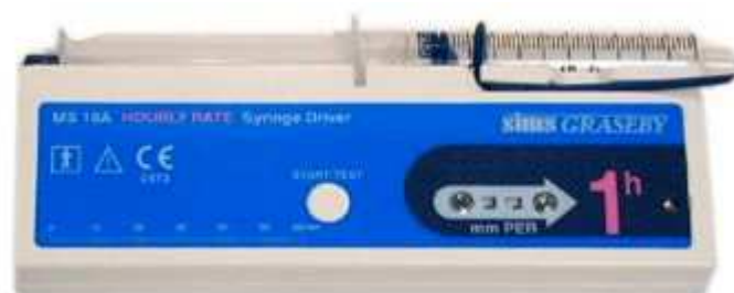
Fig. 4: Bomba infusora Grazby MS16A da Graseby Medical Limited [3].
