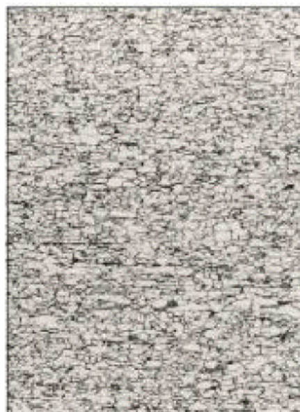
TM treatment + Acc.Cooling 1 and 2
