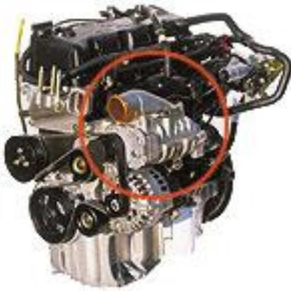
Figura 51: Motor Ford Zetec 1.0 Supercharged, com destaque no compressor.
