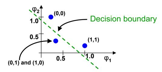
• When mapped into the feature space  $< \phi_1$ ,  $\phi_2 >$ , C1 and C2 become *linearly separable*. So a linear classifier with  $\phi_1(x)$  and  $\phi_2(x)$  as inputs can be used to solve the XOR problem.
