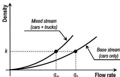
Figure 1: PCE derivation from two traffic streams with the same level of service (measured by density)
