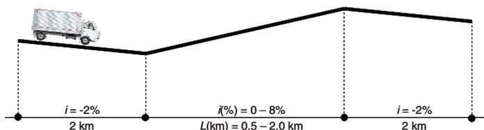
Figure 6: Profile of highway section used for PCE derivation
