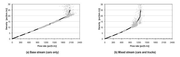
Figure 7: Flow-density curves obtained from the simulation experiments: (a) base stream, FFS = 110 km/h, L = 0.5 km, i = 0% and p = 0%; (b) mixed stream, FFS = 110 km/h, L = 0.5 km, i = 4% and p = 30%
