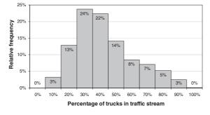
Figure 3: Distribution of observed heavy vehicle percentages in the traffic stream on the highway network used in the study
