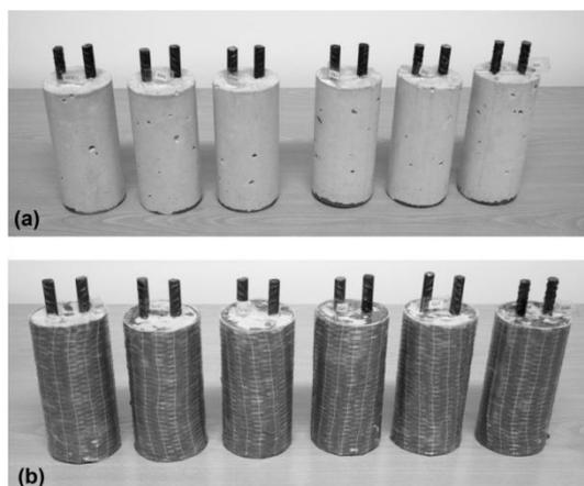
Fig. 1 – Samples: (a) without GFRP, (b) with GFRP.
