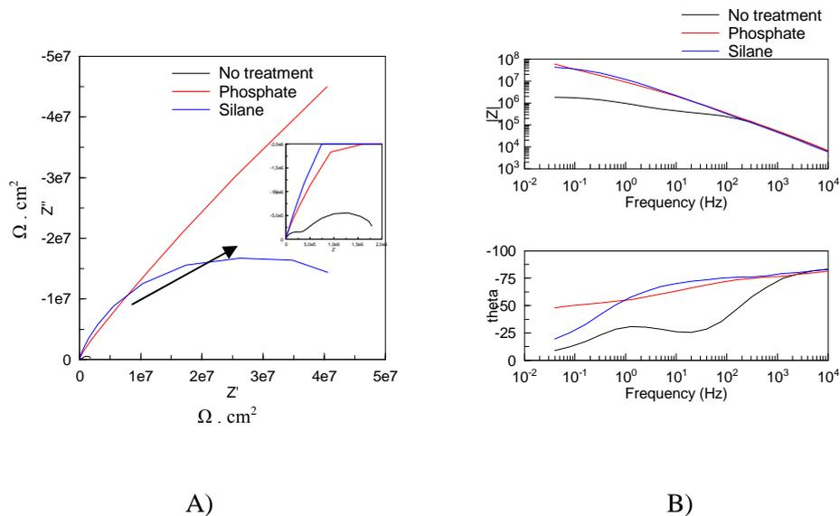
Figure 1 – Electrochemical impedance diagrams A) Nyquist and B) Bode for specimens coated with waterborne epoxy primer with different pretreatments after 3 hours of immersion in 3.5% w/w NaCl solution
