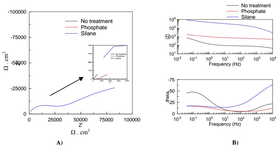
Figure 2 - Electrochemical impedance diagrams A) Nyquist and B) Bode for specimens coated with waterborne epoxy primer with different pretreatments after 530 hours of immersion in 3.5% w NaCl solution
