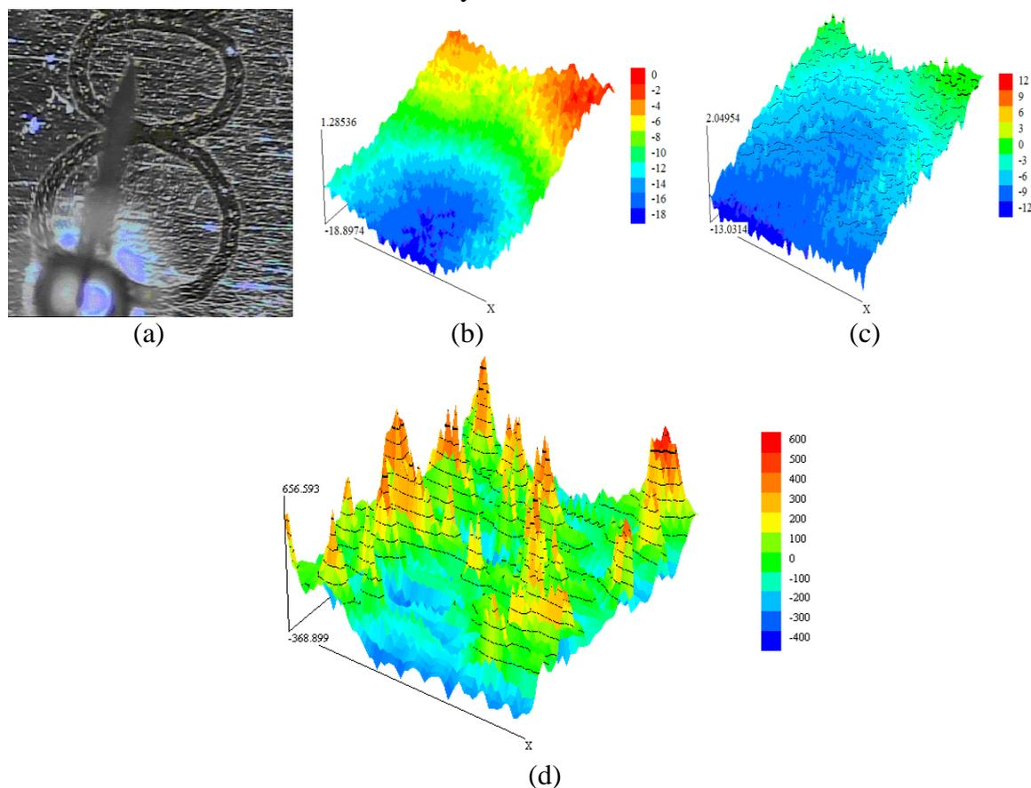
Fig. 1. Optical micro-photo of the analyzed area (a), 3D distribution of local ionic current density, immediately after immersion in PBS (b), 17h after immersion in PBS (c), under polarization conditions (d).
