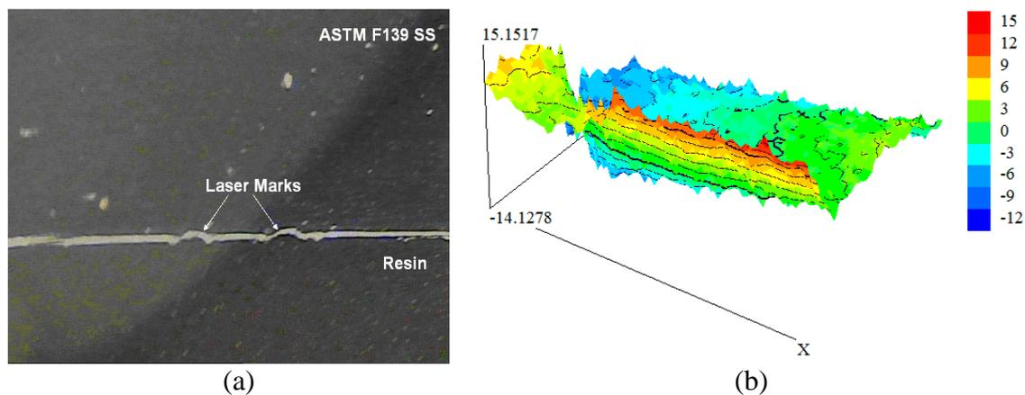
Fig.2. Cross-section optical micro-photo (a), and corresponding 3D distribution of local ionic current density (b).
