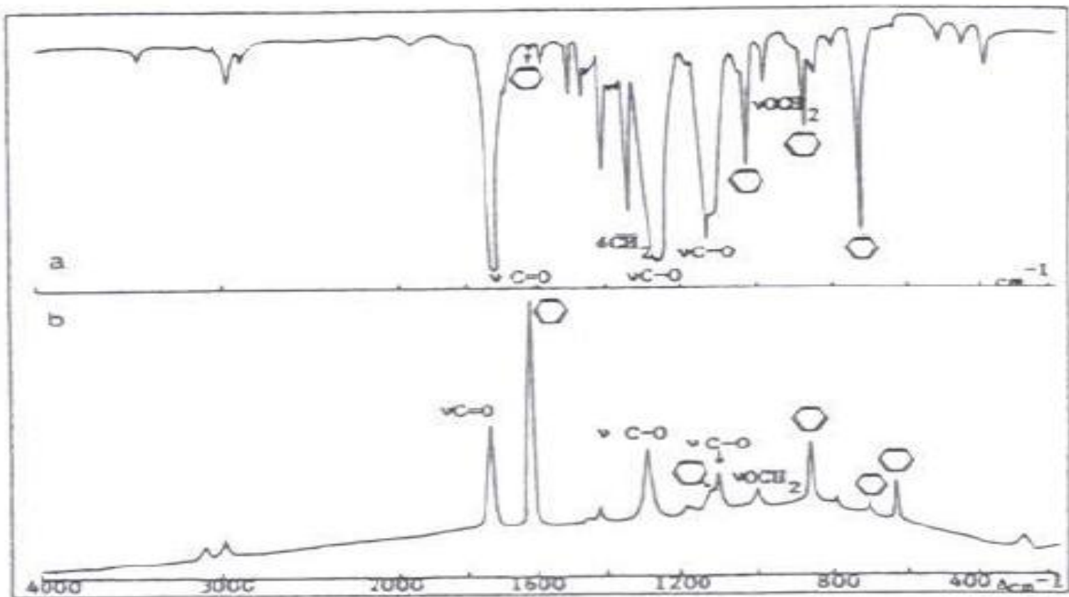
Figure 5.7. IR (a) and Raman (b) spectra of poly(ethylene terephthalate). (Reproduced with permission from reference 8. Copyright 1979 Steinkopff Verlag Darmstadt.)
