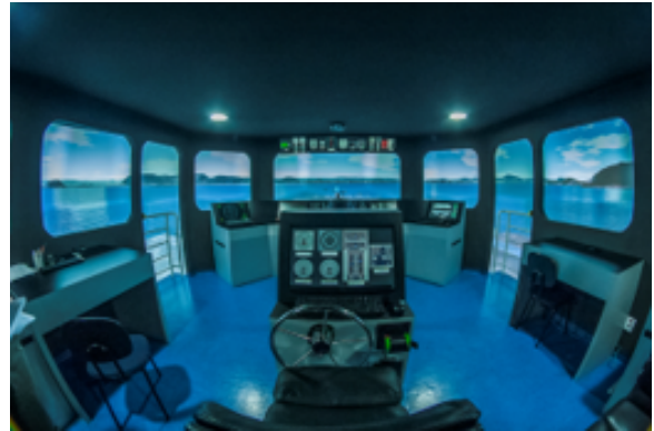
FIGURE 1. TPN-USP Full maneuvering simulator
