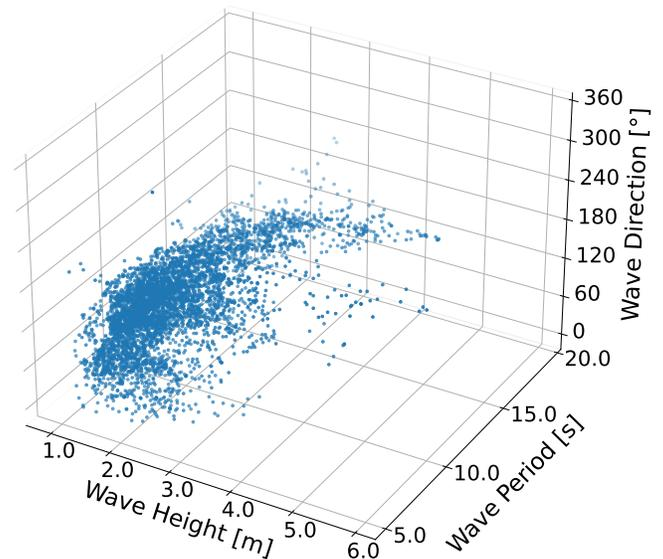
**FIGURE 2:** Distribution of  $H_s$ ,  $T_p$  and  $\beta$  in the dataset observed at a Brazil's Offshore Basin
