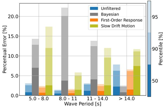
**FIGURE 15:** Percentual error  $T_p$  – Offshore Basin environmental data
