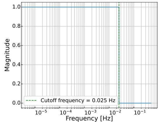
**FIGURE 4:** Filter frequency response
