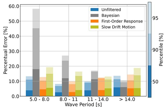
FIGURE 14: Percentual error  $H_s$  – Offshore Basin environmental data
