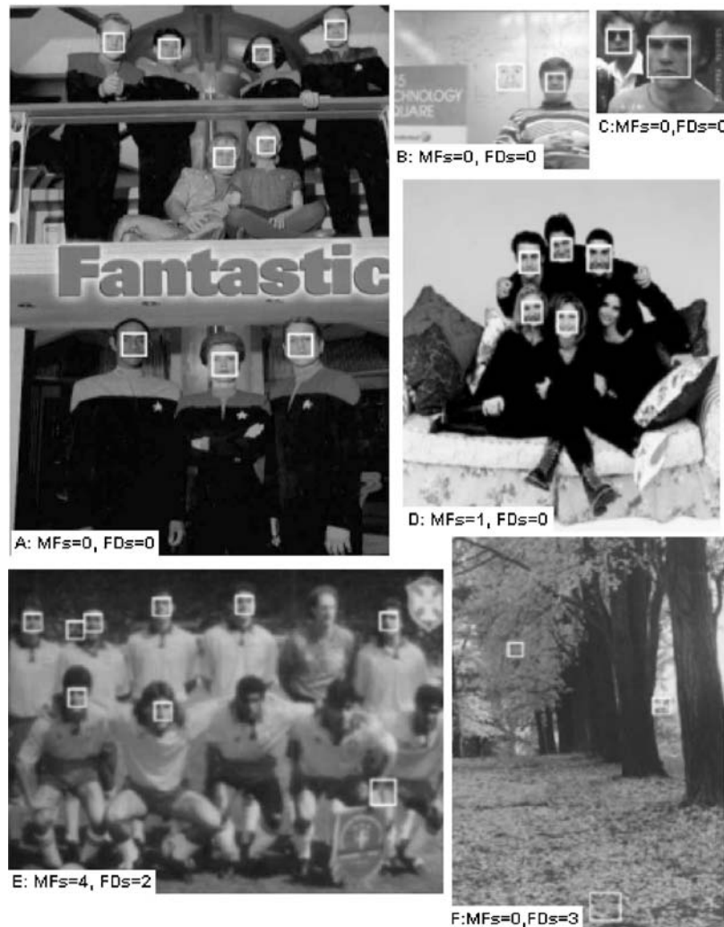
Fig. 4 Output of the system on some images of the CMU test using the SSS classifier learned with 19,000 labeled data. MFs represents the number of missed faces, and FDs is the number of false detections
