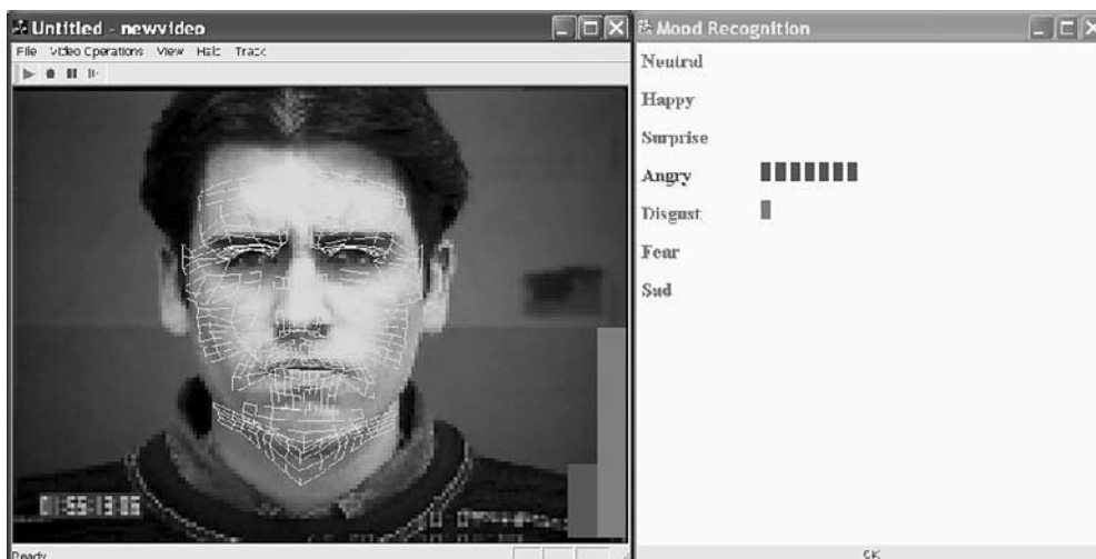
Fig. 1 A snapshot of our real-time facial expression recognition system. On the right-hand side is a wireframe model overlaid on a face being tracked. On the left-hand side the correct expression, angry, is detected (the bars show the relative probability of angry compared to the other expressions). The subject shown is from the Cohn–Kanade database
