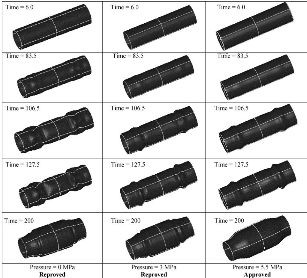
Fig. 10. FEA evolution for the THF calibration stages (time in ms).
