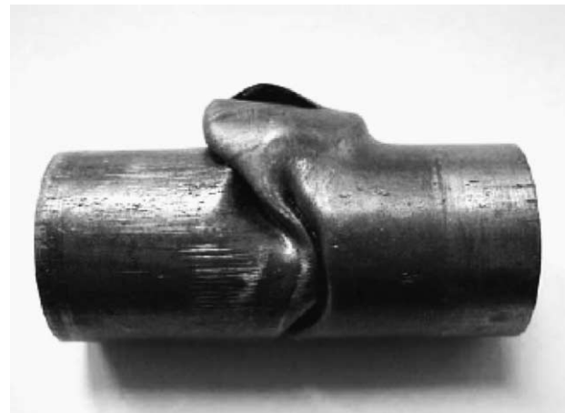
Fig. 22. THF part failure by buckling and fracture.
