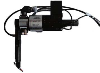
Fig. 10. Optical joining device used for coupling two different length optical fibers.
