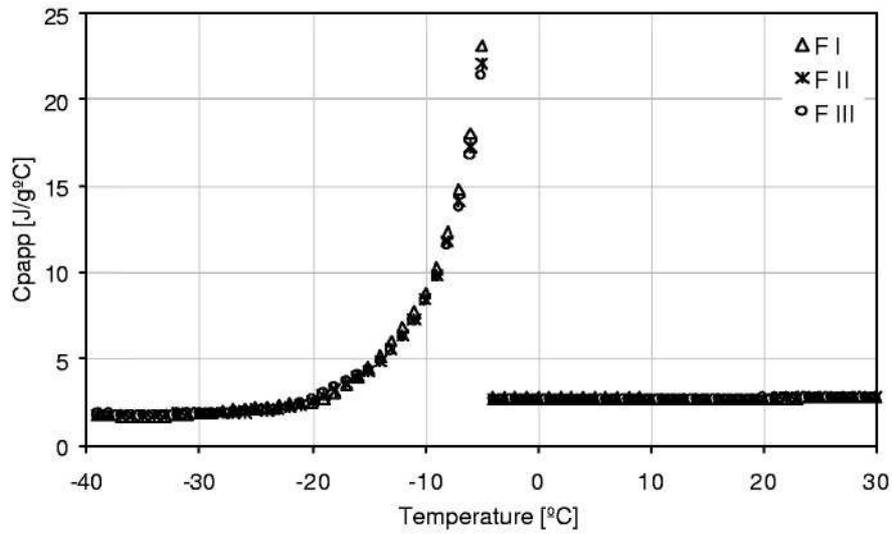
Figure 1. Experimental data of bread dough apparent specific heat for formulations with different water content. FI (A): 0.42; FII (\*): 0.43; FIII (O): 0.44.
