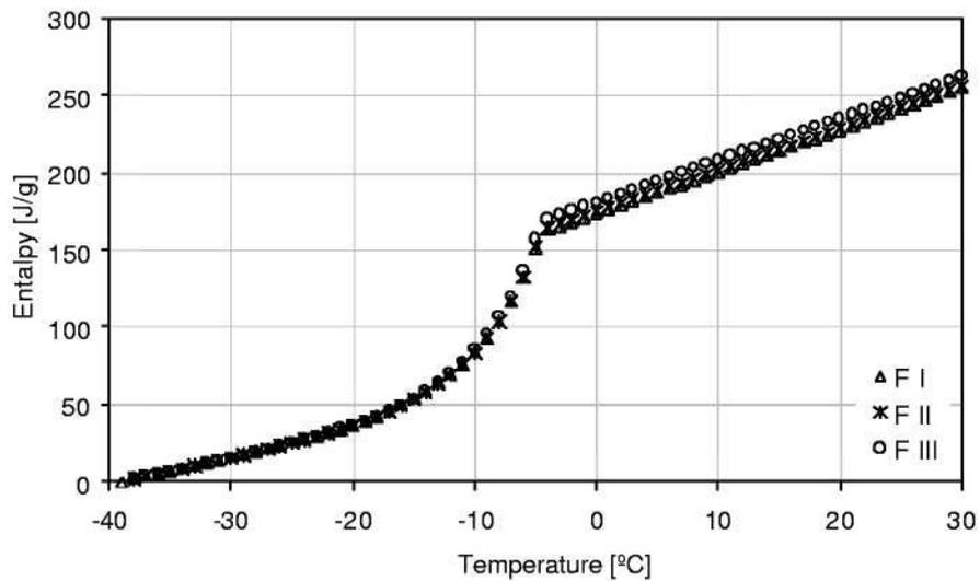
Figure 2. Experimental data of bread dough enthalpy for formulations with different water content. FI (A): 0.42; FII (\*): 0.43; FIII (O): 0.44.
