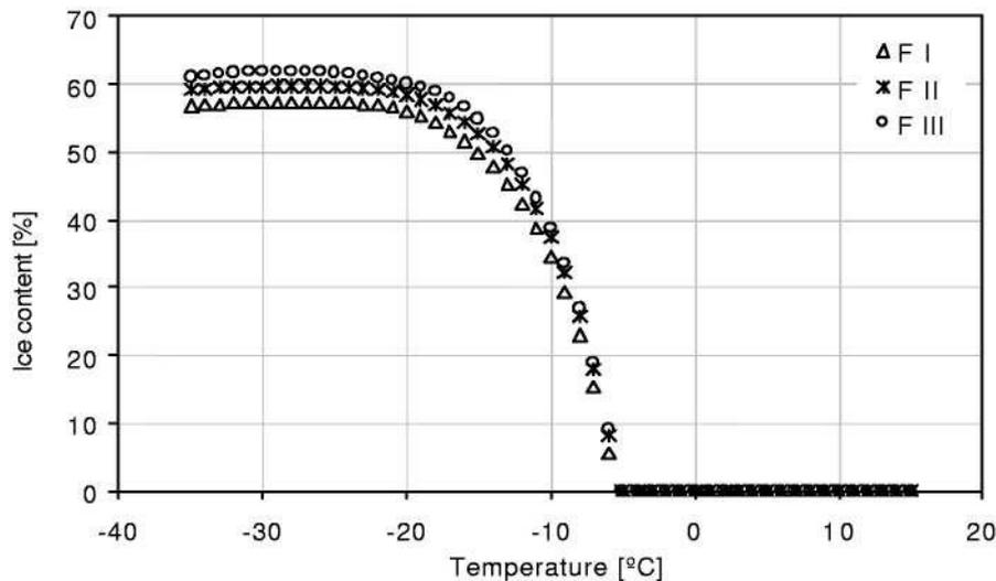
Figure 3. Ice content of bread dough for formulations with different water content. F I (A): 0.42; F II (\*): 0.43; F III (O): 0.44.
