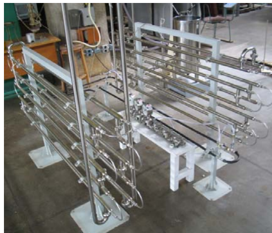
Figure 2. Photograph of the pasteurizer. Cooling heat exchanger at left and heating heat exchanger at right, with the holding tube in between.
