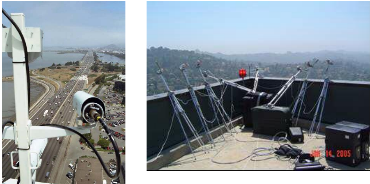
Figure 2 NGSIM Camera Setup for I-80 Data Collection in Emeryville, CA, and US 101 in Los Angeles, CA.
