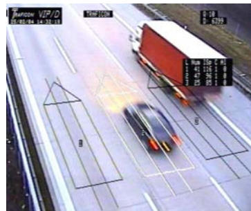
Fig. 2: Video Image Processing detectors
