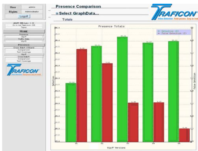
Fig. 8: Via ADEPT, different software versions are compared which makes it possible to conclude if there is improvement in the quality of the presence detection
