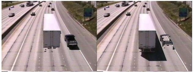
FIGURE 3 Dual-pass Otsu method for a light (left) and dark (right) vehicle.
