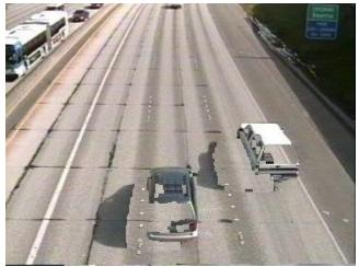
FIGURE 4 Dual-pass Otsu method in low-angle illumination.
