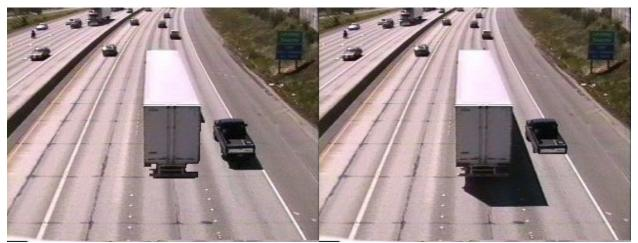
FIGURE 7 Edge subtraction and morphology method for a light (left) and dark (right) vehicle.
