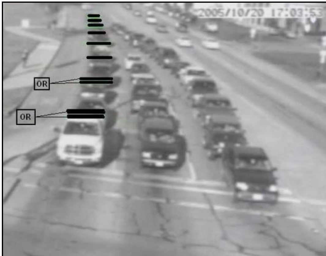
Figure 4 - Typical VIVDS Setup for Queue Detection (1)
