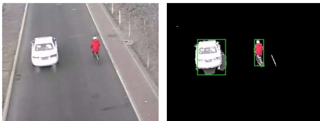
FIGURE4 Moving objects detection results (a) Source frame; (b) Foreground moving objects
