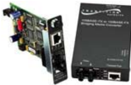
Figure 3-13: 100 Base-T to 100 Base-FX Media Conversion (NW04, CIVL02)
