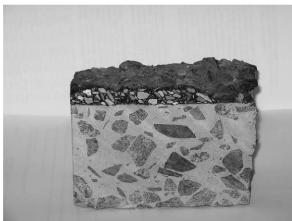
Figure 5. Core from UTW of SP-280.
