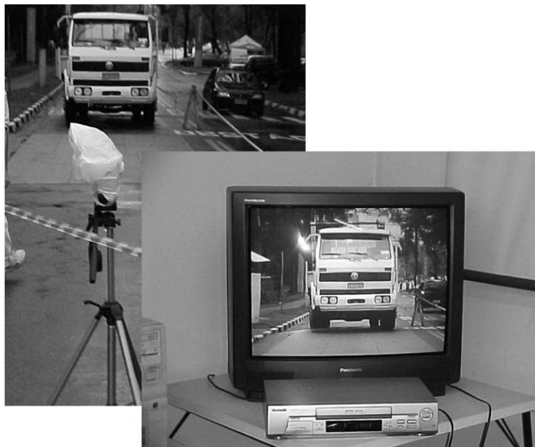
Figure 11. Dump truck video records to access the exact tires' position over UTW slabs.
